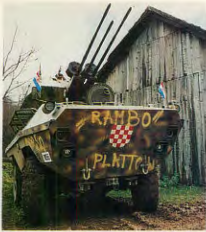
Croatian BOV-3 SPAAG at front line near Karlovac shows "custom" paint job, colors of Croatian army. Mounting three 20mm guns, BOV-3 can engage aerial targets up to 1,500 meters.
